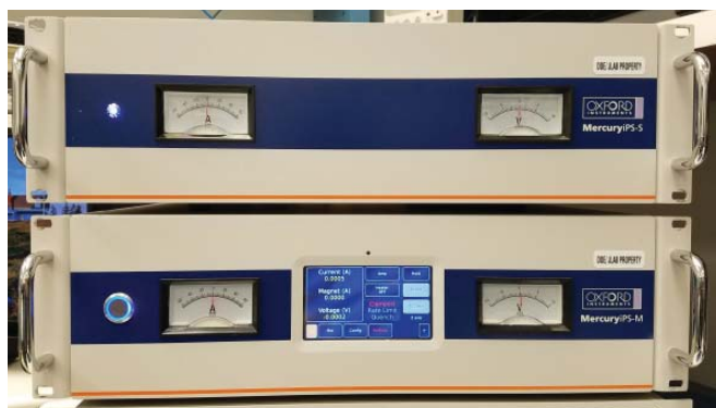
FIG. 1. Oxford Instruments Mercury iPS power supply, configured with master shown on bottom and one slave on top.
